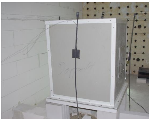
Valve Fire Shelter before start of test
