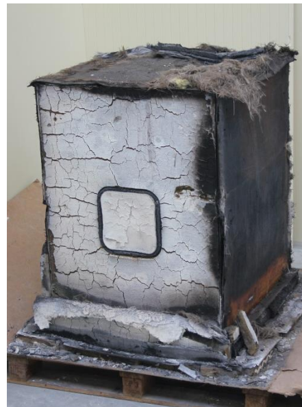
Valve Fire Shelter after test >60 min. at 1200°C /2000°F
