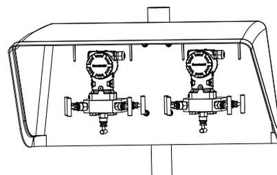
Two differential pressure transmitters with BM-manifolds, mounted on an optional mounting plate to an external pipe stand. Connection of the impulse and vent lines on the rear (horizontally).
