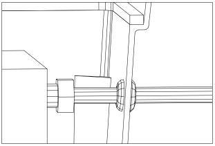
A good seal can only be guaranteed if the entire sealing surface is in close contact with the wall.
