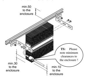
The brackets in zinc coated steel and fixing bolts illustrated above are included with the heater.
