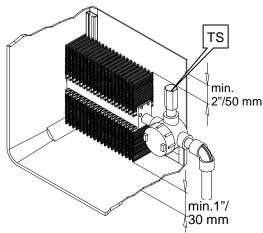
**Note:** The convection is about 20% less at vertical installation. Due to earlier switching of the thermostat the effective heating power may be lower.
