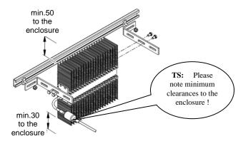
The brackets in zinc coated steel and fixing bolts illustrated above are included with the heater.
