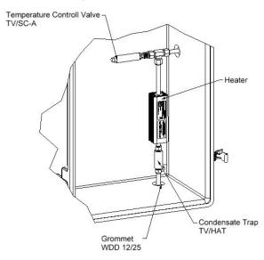
Steam heater, controller and trap.
