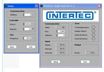
Up to 31 TC D controllers can be connected to the RS485 interface. All controllers can be operated and monitored from a PC.
