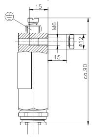
Optionally, the supplied bolt M6x25 or a smaller through-bolt can be used.
