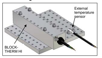
The Blocktherm heater transmits its' heat through conduction. Therefore when installed, it shall be firmly attached to an even surface which conducts heat well (metal). The heater should be fastened with 4 screws.
