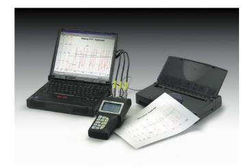
The ServiceMaster is a multi-channel hand meter for the simultaneous measuring of important hydraulic values:
