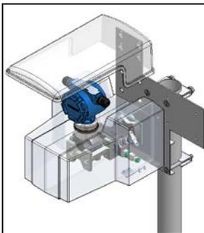
MESC Box with manifold and Rosemount-transmitter 3051 S mounted underneath SHADE SD 22 and attached to a 2" pipe stand by means of a mounting system.
