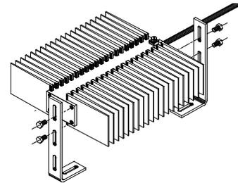
The brackets and mounting bolts illustrated above are included with the heater.
