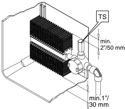
**Note:** The convection is about 20% less at vertical installation. Due to earlier switching of the thermostat the effective heating power may be lower.
