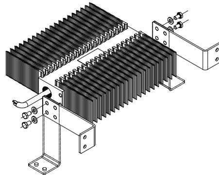
The MB or MW mounting brackets can be ordered as options.
