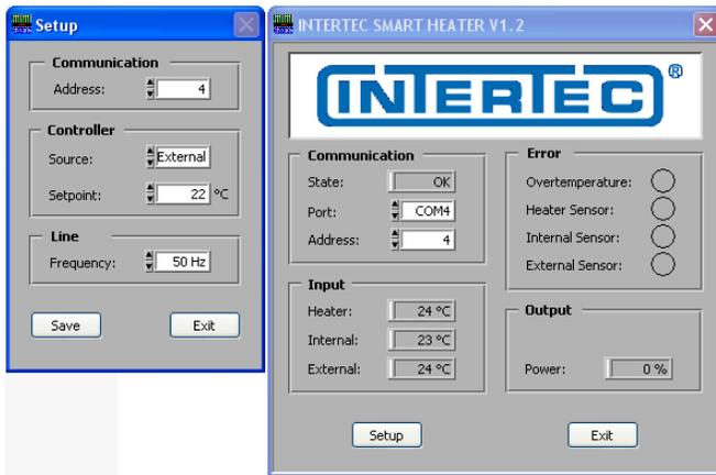
Up to 31 TC D controllers can be connected to the RS485 interface. All controllers can be operated and monitored from a PC.
