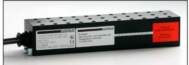
CP BLOCKTHERM is a metall block that has an electric heating cartridge and a temperature sensor for electronic temperature limitation integrated.
