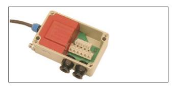
The controller consists of an electronic section with microprocessor, completely encapsulated in silicone, and a terminal section with EEx e terminals. The controller has three analogue inputs:
