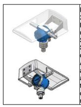
Rosemount transmitter 3051... or Endress and Hauser F12/T12 mounted underneath
